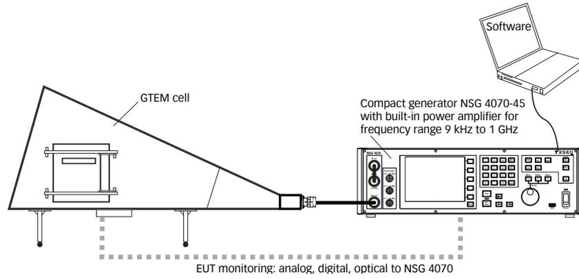
Figure 50: Setup with GTEM cell and NSG 4070-45
