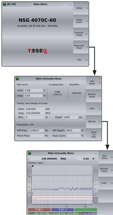
The softkey **Results** shows the current test result which can be investigated by turning the rotary knob. The red curve shows the voltage on the analog EUT monitoring input, and is related to the left axis. Other EUT monitoring events are displayed above the graph with different colors.
