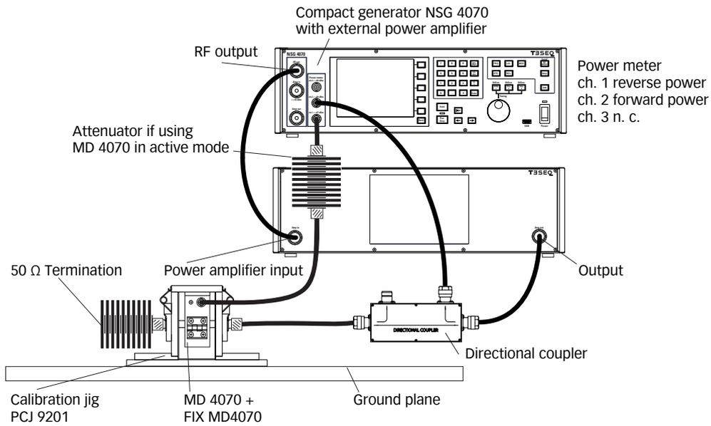
**Figure 37: Probe calibration setup with external power amplifier**
