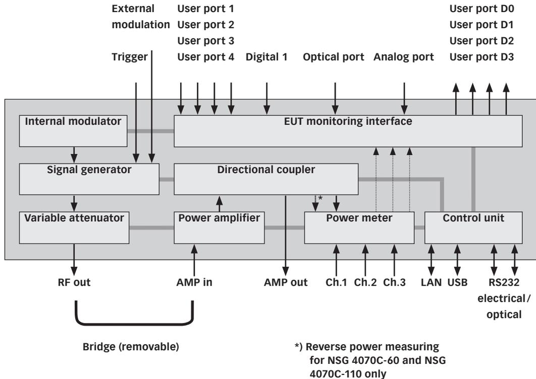
Figure 1: Block diagram of NSG 4070 with internal power amplifier
