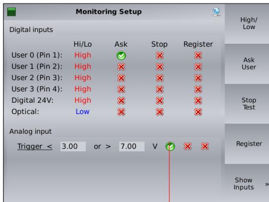
The action in case of a trigger event (EUT failure) can be set either to register the occurrence of the event (lowest priority), to stop the test, or user decision (highest priority) using the corresponding softkeys (see chapter 4.5.2 for details).
