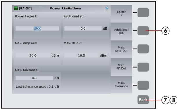
6. Press **Additional Att.** and change this value to 0 dB except the power amplifier is >100 W and MD 4070 is switched to the active mode. This would be require at least 10 dB.
