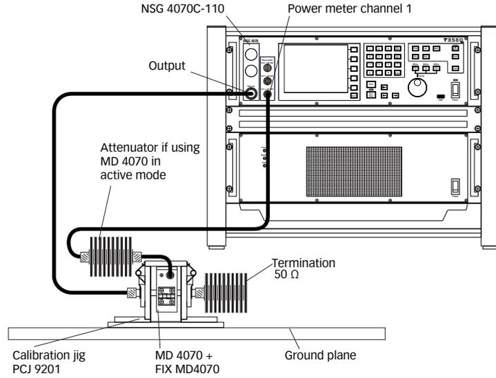
**Figure 36: Probe calibration setup with internal power amplifier (e.g. NSG 4070C-110)**
