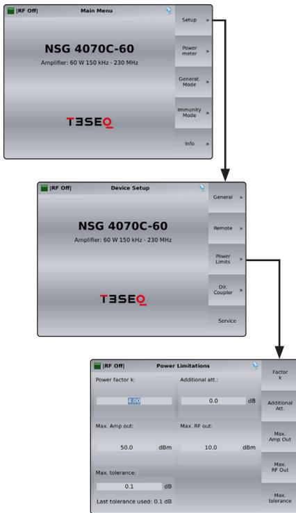
**Power Limits** allows the user to set system limits. **Factor k** is a power limitation factor as described in the ISO 11452-4 standard. The default value is 4. (See chapter 8.3.7 for more information.)
