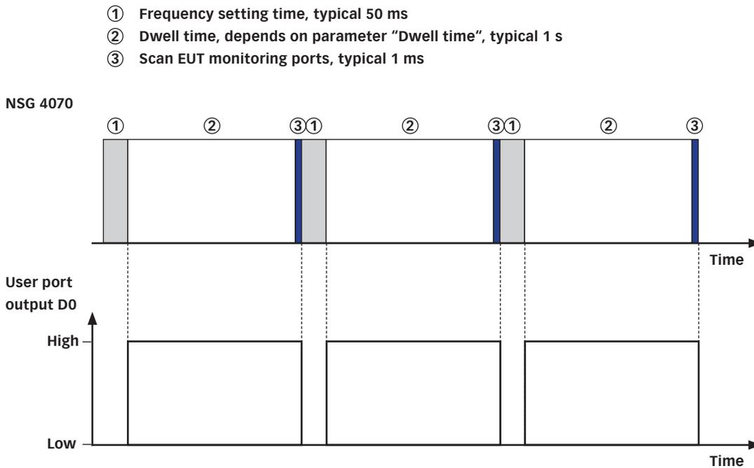
Figure 5: Timing of User port D0 output in "auto" mode
