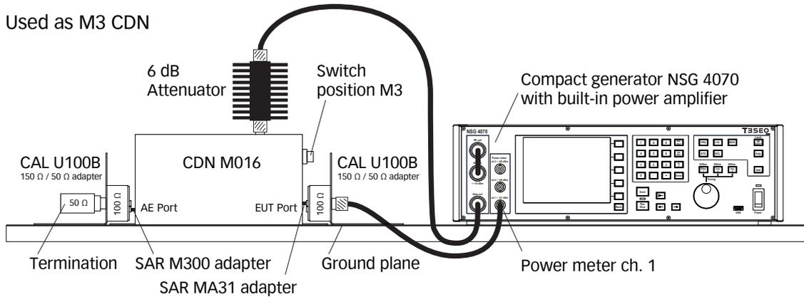
Figure 13: Test setup calibration with CDN M016 (switchable M2/M3)
