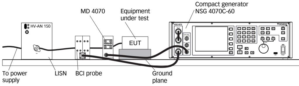
**Figure 40: BCI test setup with current monitoring probe with internal amplifier (e.g. NSG 4070C-60)**
