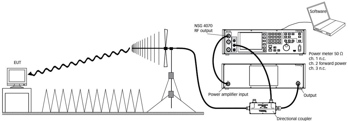
Figure 49: Setup with antenna and NSG 4070 with external power amplifier
