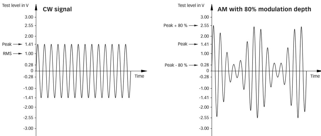
**Figure 8: Amplitude modulation**
