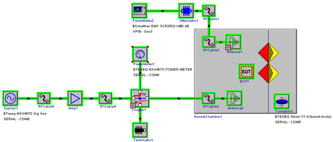
Figure 52: CIS test house software configuration of a reverberation chamber setup with NSG 4070
