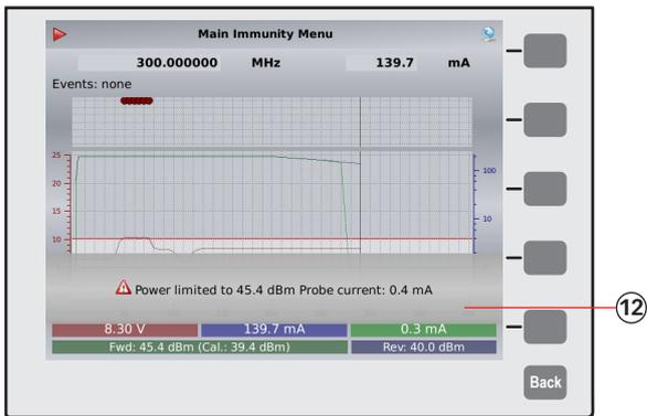
12. Example of a message in case of power limitation (For example means a k factor of 4: An increase to four times the calibrated forward power isn't enough to reach the target level. There will be no increase above this limitation.)
