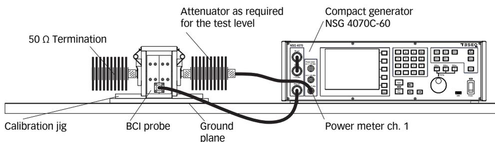
Figure 30: BCI calibration setup with internal power amplifier (e.g. NSG 4070C-60)
