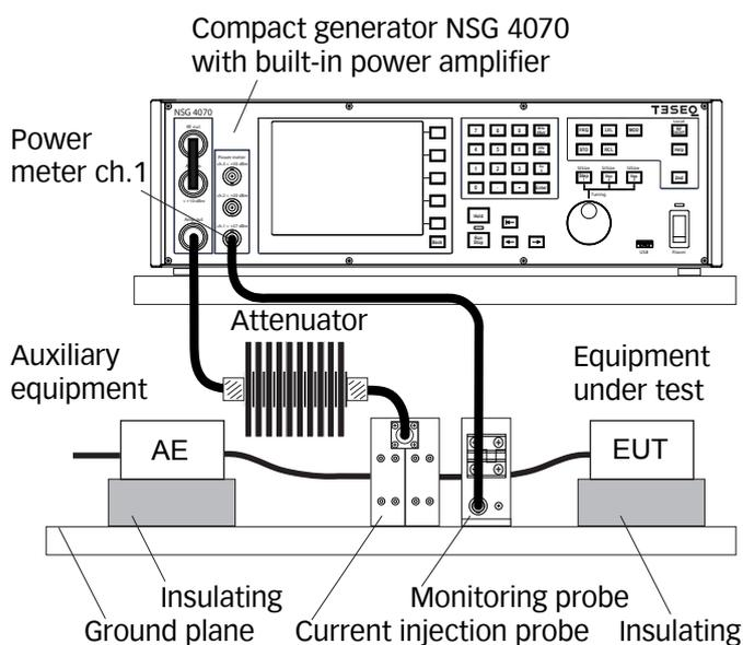
Figure 24: Test setup with EUT according IEC/EN 61000-4-6 with current injection probe and monitoring probe
