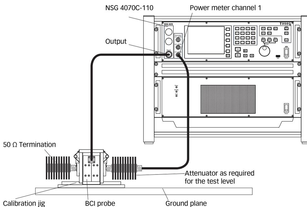
Figure 31: BCI calibration setup with internal power amplifier (e.g. NSG 4070C-110)
