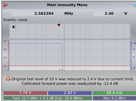
Testing with a monitoring probe requires a coupling device such as an EM clamp or CIP with selected "With probe" BCI testing requires "Substitution with monitoring device" or "Closed loop" for including a monitoring probe.
