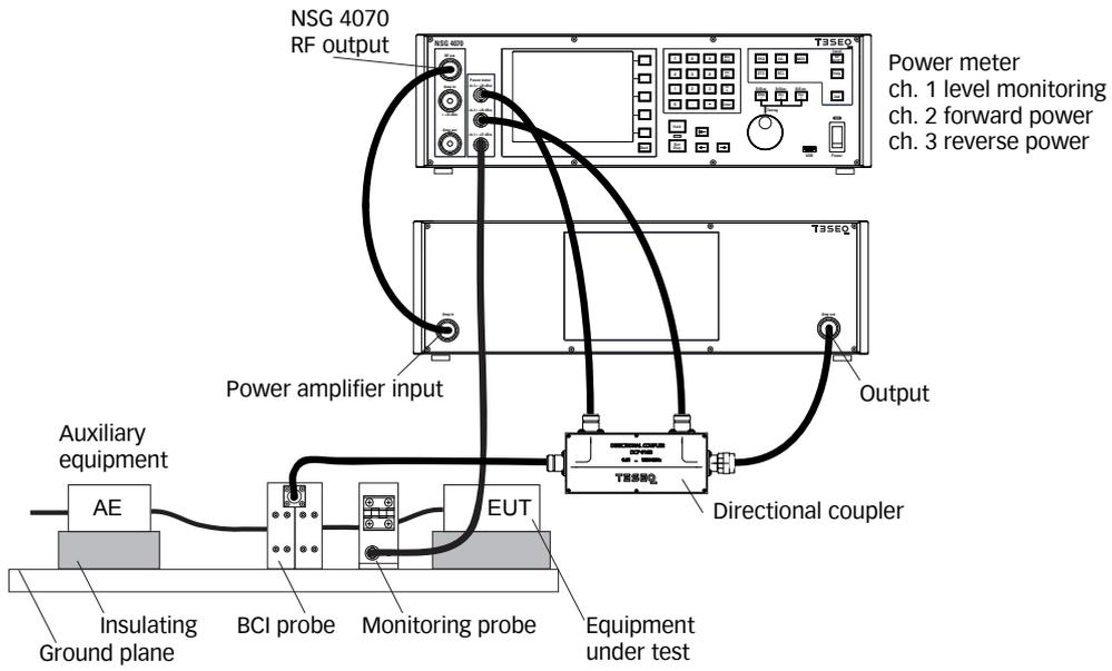
Figure 42: BCI test setup with current monitoring probe with external amplifier
