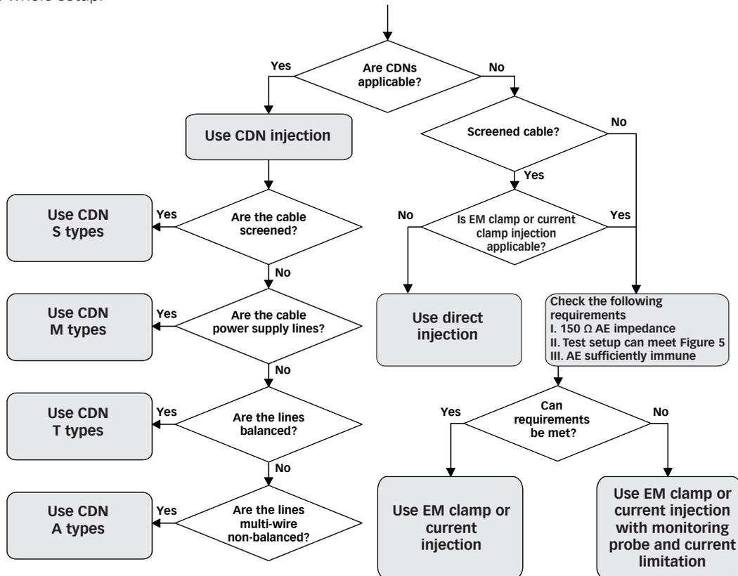
Figure 9: Rules for selecting the injection method (Chapters 7.2 to 7.5 refer to the IEC/EN 61000-4-6 standard.)
