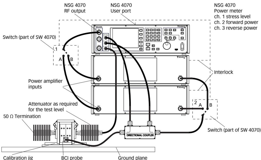
Figure 34: BCI calibration setup with internal and external power amplifier (Mix operation)
