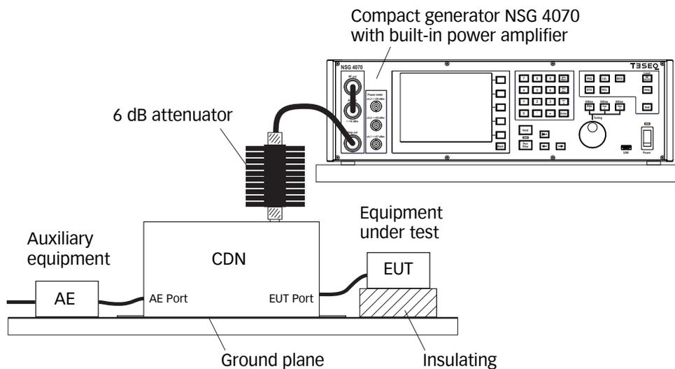
**Figure 16: Test setup with EUT**
