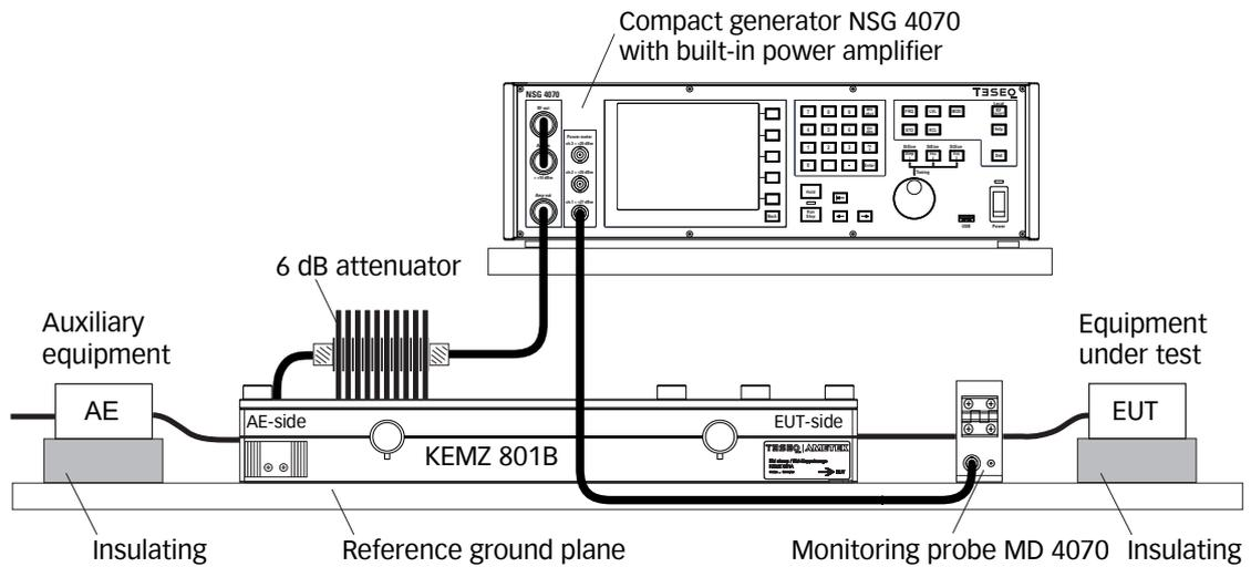
**Figure 19: Test setup with EUT according IEC / EN 61000-4-6 with EM clamp and monitoring probe**
