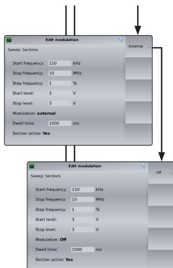
Using the modulation input on the rear panel and selecting **(Mod: Ext.)** allows a sinusoidal signal with 1 V peak to peak to get a modulation factor of 100 %.
