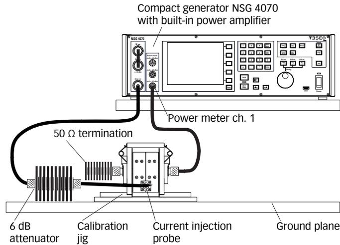
**Figure 21: Test setup calibration with current injection probe in a 50 Ω system**
