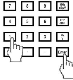
Select the desired field with the softkey, do the selection or type in the new parameter with help of the keypad or connected keyboard. Confirm the input with the relevant soft or hardkey.
