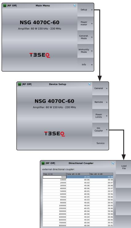
The softkey **Load File** offers the import function for the coupling attenuation calibration factors of the external directional coupler.
