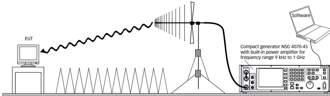
Figure 48: Setup with antenna and NSG 4070-45
