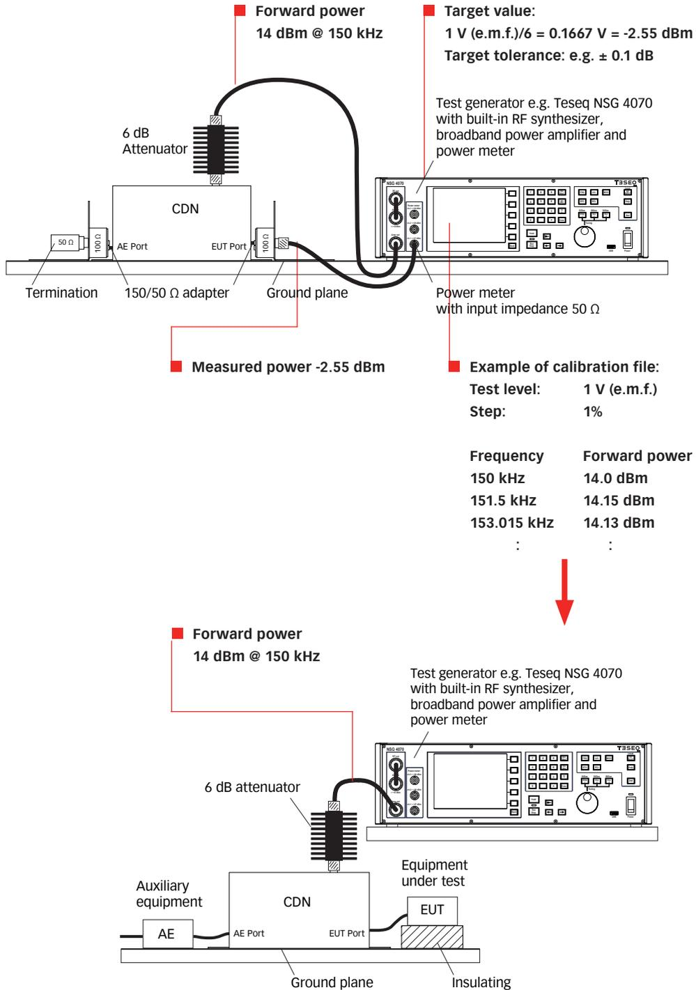
Figure 7: Example for test level setting, relation between test level and measured level (The influence of the modulation is neglected in this sample.)
