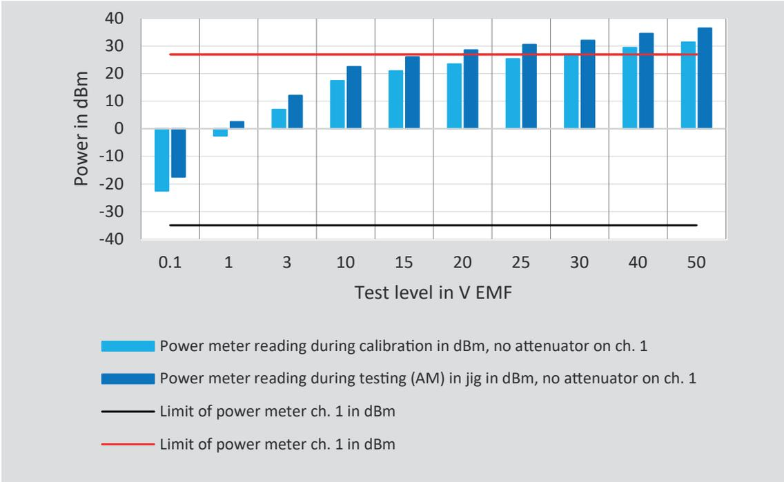
Figure 10: Power meter channel 1 typical readings without attenuator
