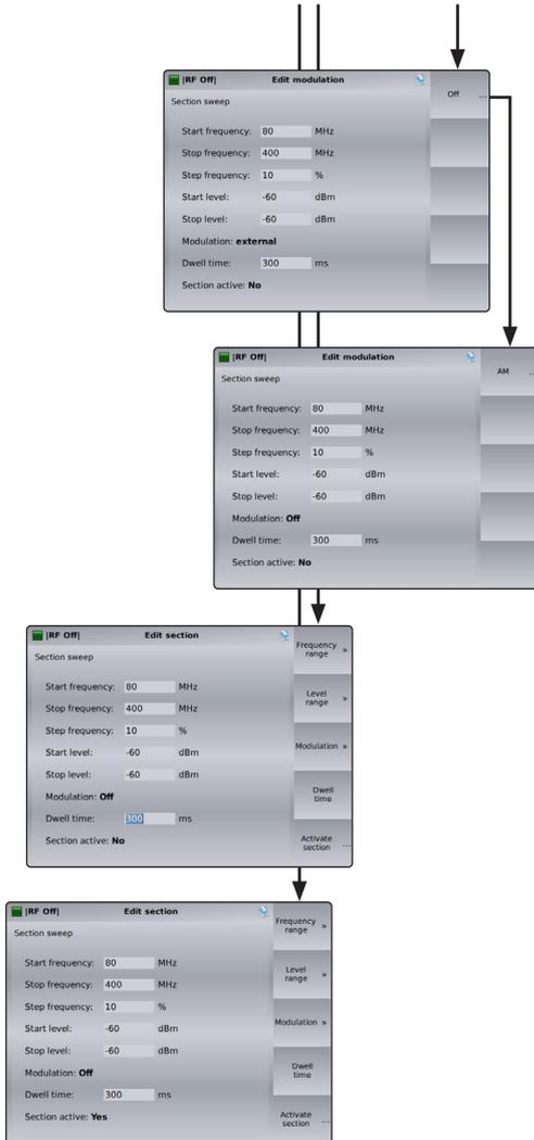
Using the modulation input on the rear panel and selecting **(Mod: Ext.)** allows a sinusoidal signal with 1 V peak to peak to get a modulation factor of 100 %.
