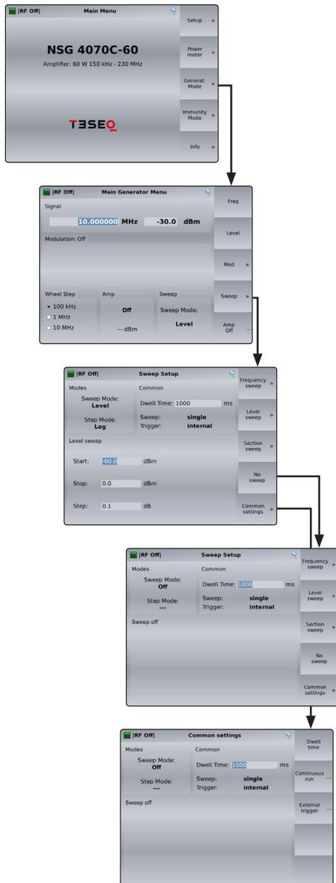
The Generator mode offers frequency, level or section sweep modes.
