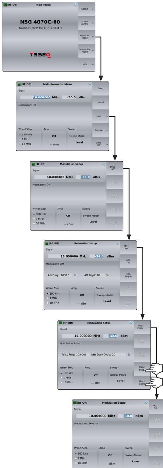
Modulation can be set to AM (amplitude modulation), PM (pulse modulation), external or off. The modulation can be changed by pressing the upper softkey.
