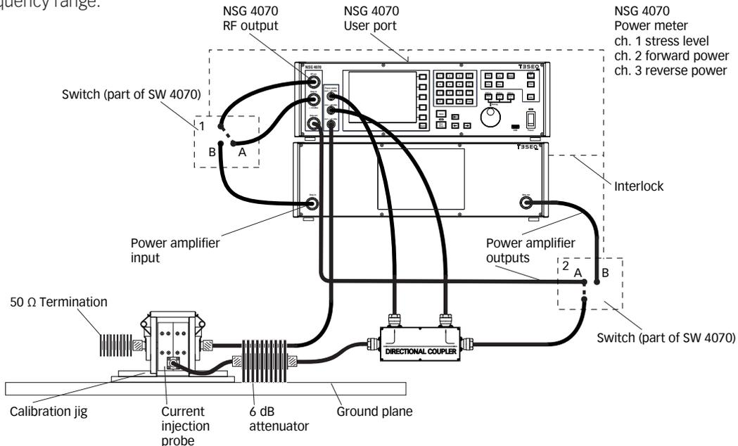
**Figure 22: Test setup calibration with current injection probe in a 50 Ω system, 2 amplifiers**
