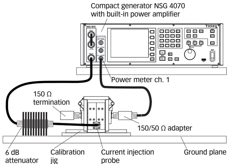
**Figure 20: Test setup calibration according IEC/EN 61000-4-6 with current injection probe**
