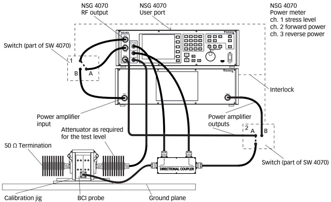
Figure 33: BCI calibration setup with two external power amplifiers
