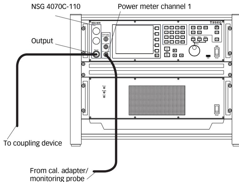
Figure 28: Setup with NSG 4070C-110
