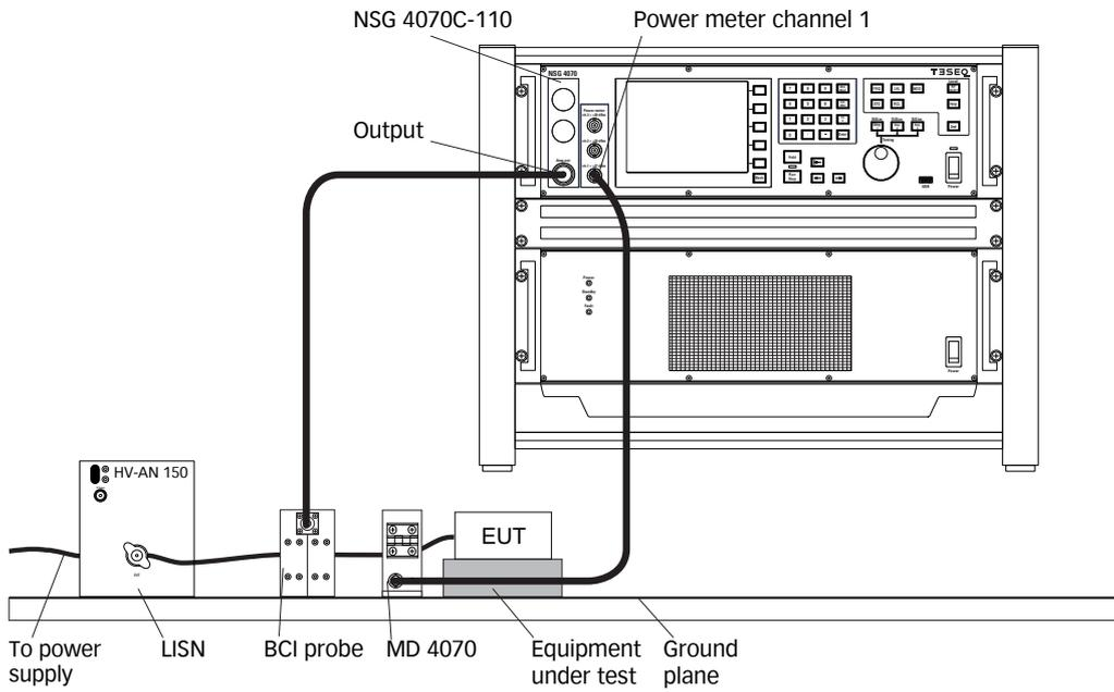
**Figure 41: BCI test setup with current monitoring probe with internal amplifier (e.g. NSG 4070C-110)**
