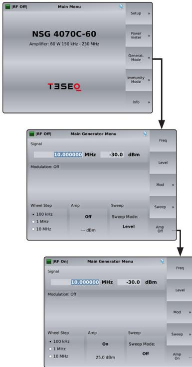
Every NSG 4070 model except the 4070-0 includes an internal amplifier. The amplifier is turned on by pressing the softkey **(Amp On)** in the Main Generator menu. The drive level, or signal generator output level, is limited to 0 dBm when the amplifier is in use. The amplifier output level (forward power) and the signal generator level (amplifier module drive level) are displayed.
