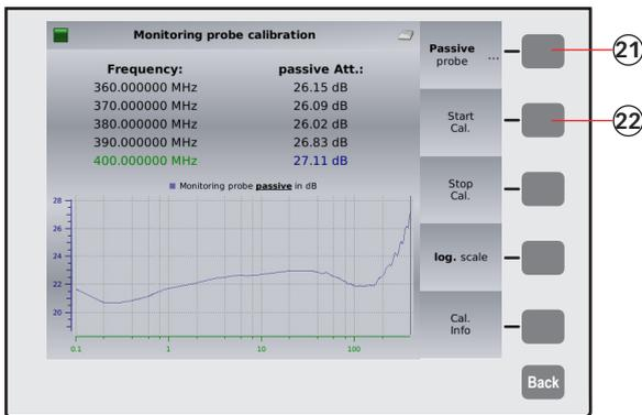
21. Select **Passive probe** if using MD 4070 passive. Select **Active probe** if using MD 4070 active.
