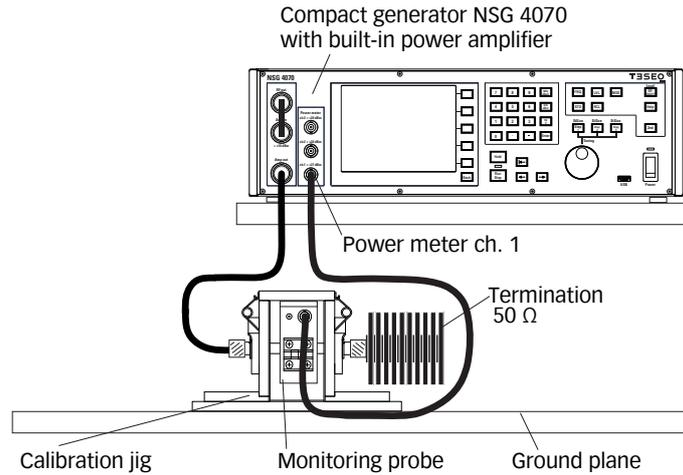
**Figure 25: Calibration setup of the monitoring probe**
