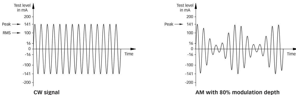
Figure 29: Amplitude modulation with peak conservation
