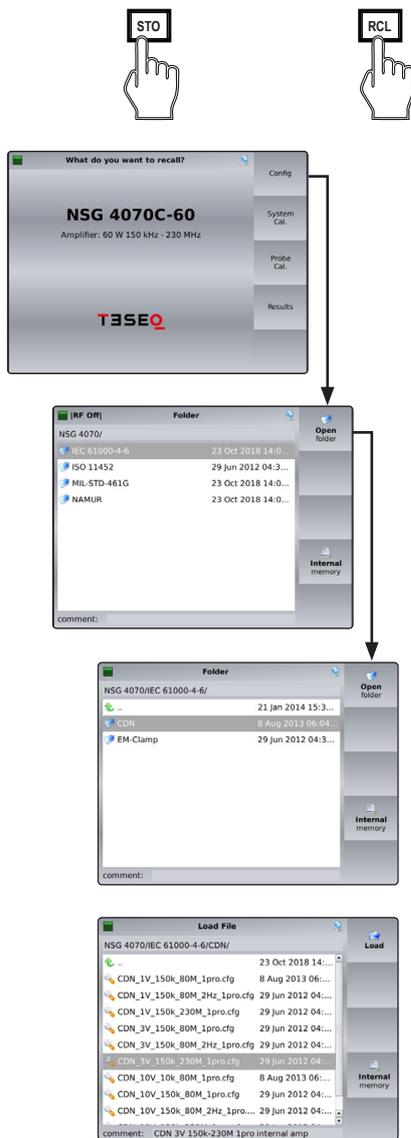
In general, the hard keys **STO** and **RCL** allow the user to store and to recall configurations, system calibration data, probe calibration and results.
