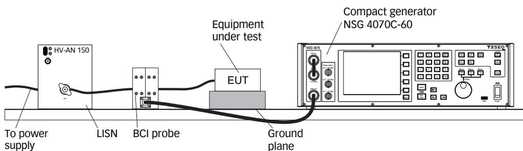
**Figure 38: BCI test setup without current monitoring probe with internal amplifier**
