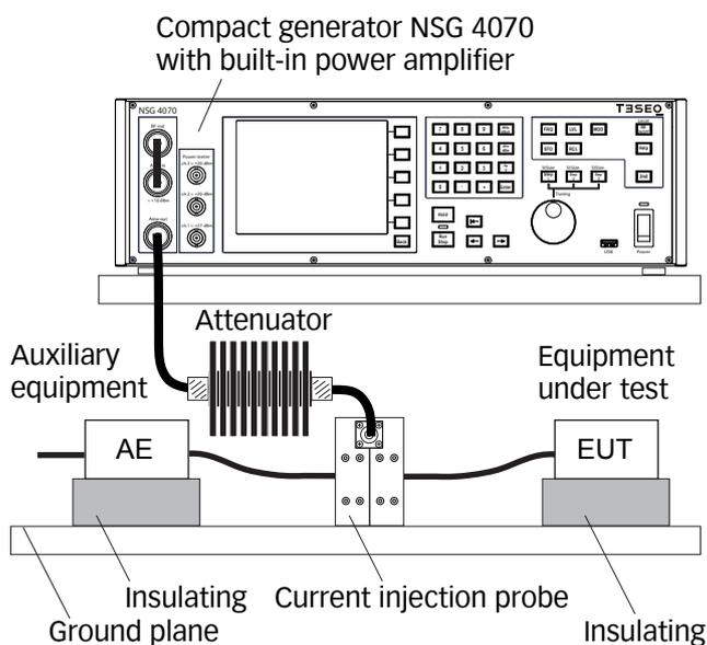
Figure 23: Test setup with EUT according IEC/EN 61000-4-6 with current injection probe
