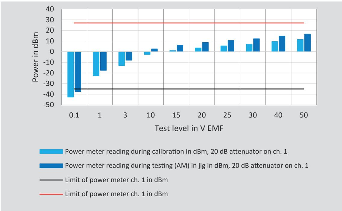
Figure 11: Power meter channel 1 typical readings with 20 dB attenuator
