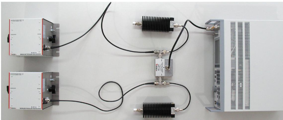
Figure 44: NSG 4070C-80 + SET 4001 (“line-to-line” coupling)
