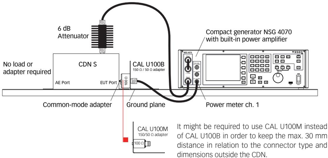
**Figure 15: Test setup calibration with CDN S**
