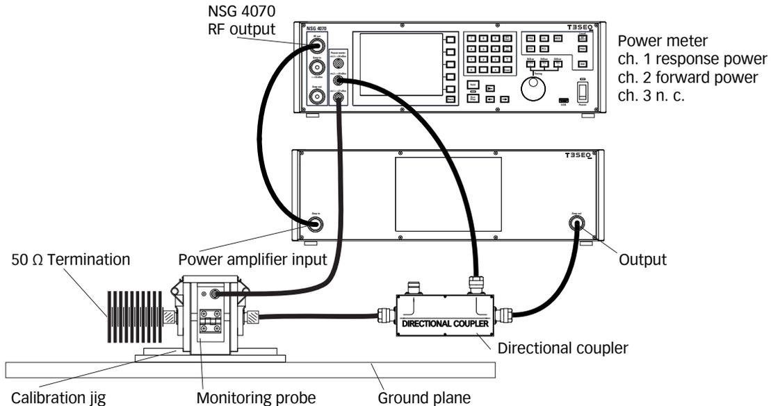
**Figure 26: Calibration setup of the monitoring probe with external power amplifier and directional coupler**
