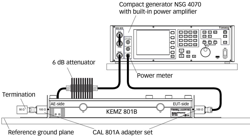
Figure 17: Test setup calibration according IEC/EN 61000-4-6 with EM clamp
