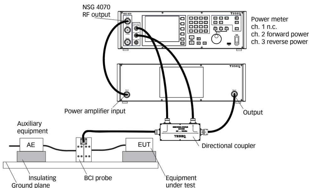
**Figure 39: BCI test setup without current monitoring probe with external amplifier**
