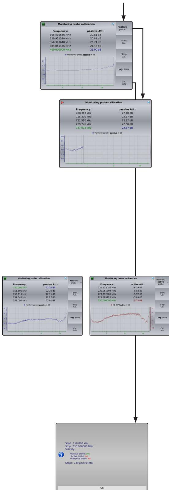
The calibration result can be observed by turning the rotary knob. The blue curve shows the probe calibration result in the passive mode, which is related to the left axis. The red curve shows the result in the active mode, which is related to the right axis.
