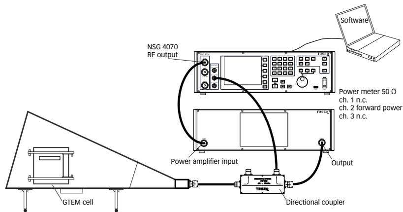
Figure 51: Setup with GTEM cell and NSG 4070 with external power amplifier
