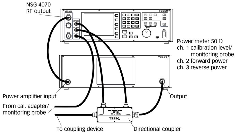
Figure 27: Setup with external power amplifier and directional coupler
