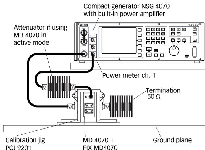
Figure 35: Probe calibration setup with internal power amplifier (e.g. NSG 4070C-60)
