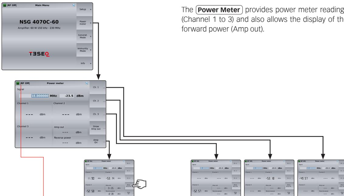
The **Power Meter** provides power meter readings (Channel 1 to 3) and also allows the display of the forward power (Amp out).
