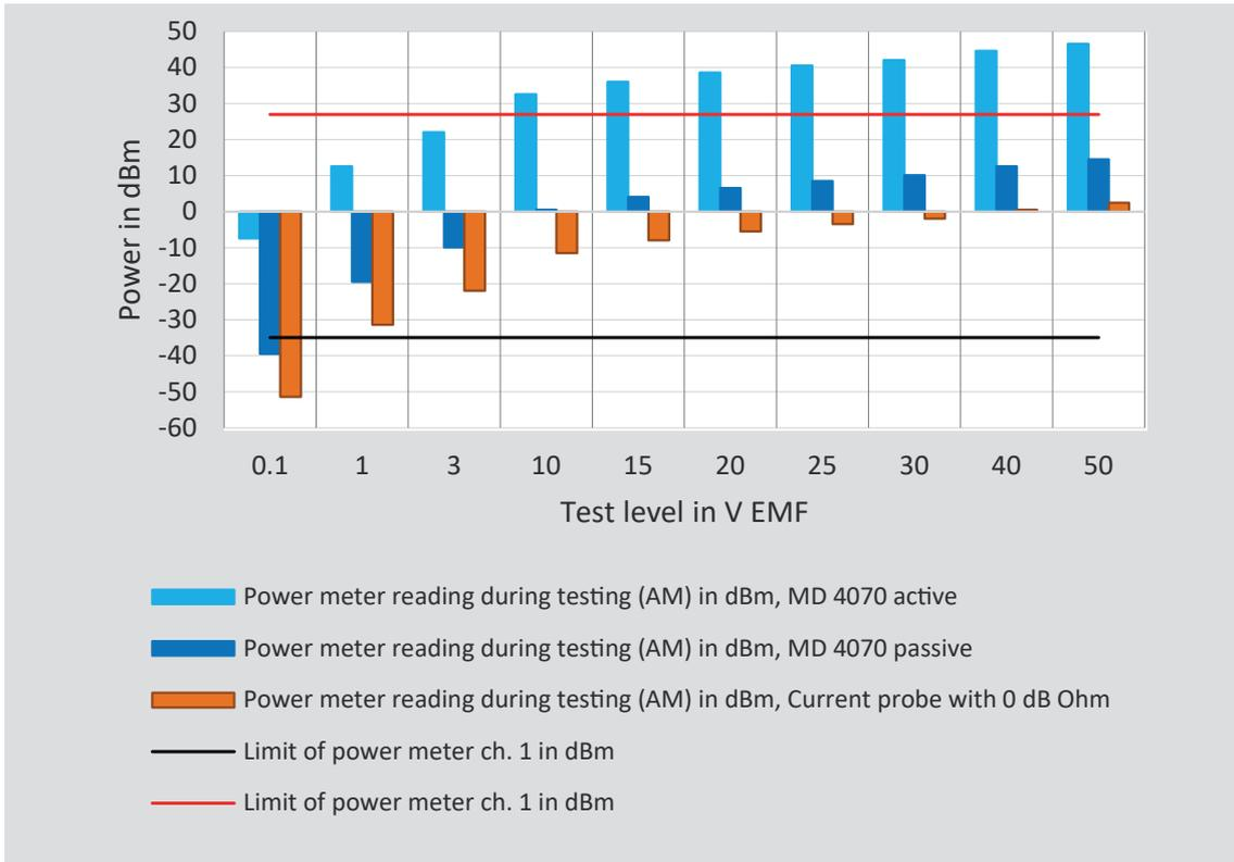
**Figure 12: Power meter channel 1 typical readings with using the current probe**
