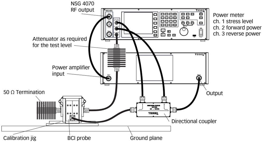
Figure 32: BCI calibration setup with external power amplifier
